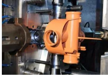
Sewage Chamber Mould
